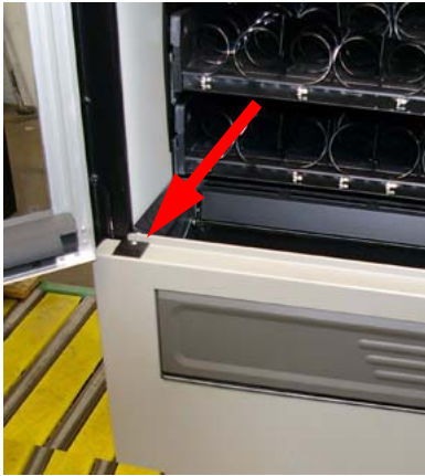
Install two 1812020 RAMP - DOOR on the top of delivery bin replacing the original and installing new part on the left side of the the delivery bin using two 6402064 RIVET-POP-ALUMI-NUM-.125 DI. There will be a new RAMP on both the right and the left sides.
