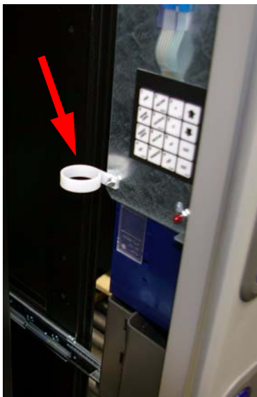
Install 3631171 CLIP-HARNES-1.50 on the lower area of the coin mech bracket.
