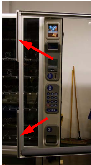
With the glass door open, install 4112095 TAPE - FOAM on the inside lip of the front glass door in two places.
