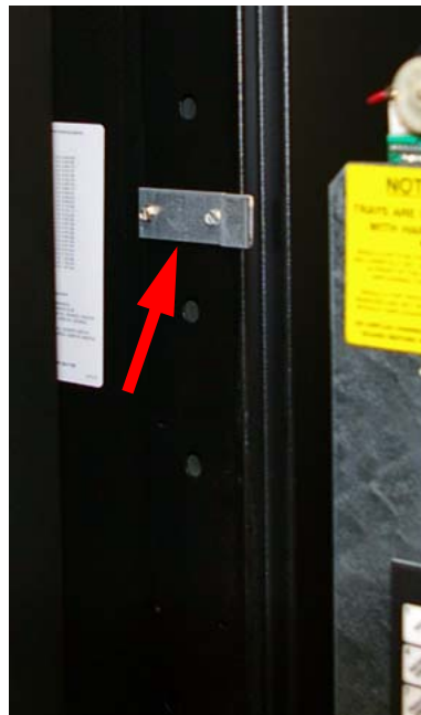
Install 1815095 BRACE-MONETARY STABILIZER on the inside right wall of the monetary section. Use two 3157060 SCREW #8-32X.31 HEX HD.
